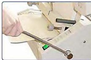
**Step Six** – If your binder has the Paper Grain Opener (“PGO”), run it across the book spine. The PGO micro-slits the paper fiber and is especially beneficial when binding coated stock.
