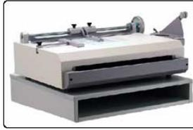
Step Three - Building the hard case. The Fastbind hard cover maker can make a cover in less than two minutes.
